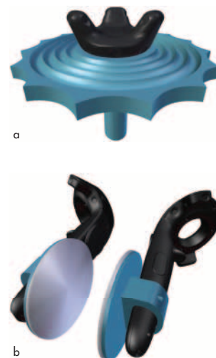
Fig. 4. (a) A revision of the resonator from our first prototype with continuous grooves and surfaces. (b) A new Hyperreal Instrument design based on the use of magnets to incorporate force feedback in a virtual instrument. (© Anil Çamcı)
